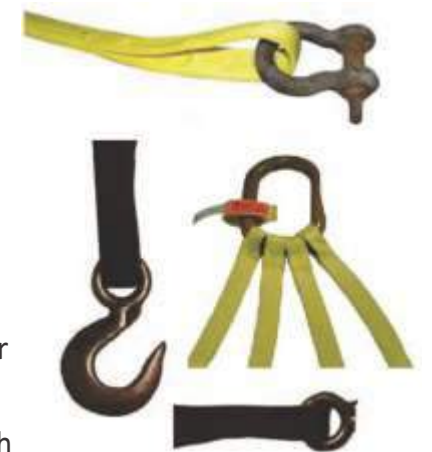
Damaged or Pitted Fittings
