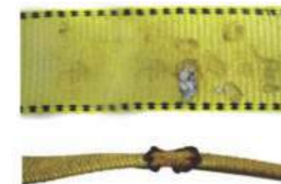
Sling Weld Splatters and Charring/Melting
